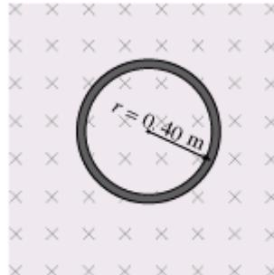
The magnetic field then changes to a value of  $0.10 \text{ T}$  in the opposite direction in  $2.10 \text{ s}$ . What is the average emf induced in the coil during the time that the magnetic field was changing?
